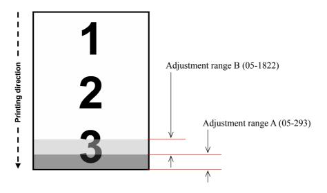
(a) Enter adjustment mode [05]. Change the value for code [293] to correct the transfer roller bias output at the trailing edge of the paper in adjustment range A.
